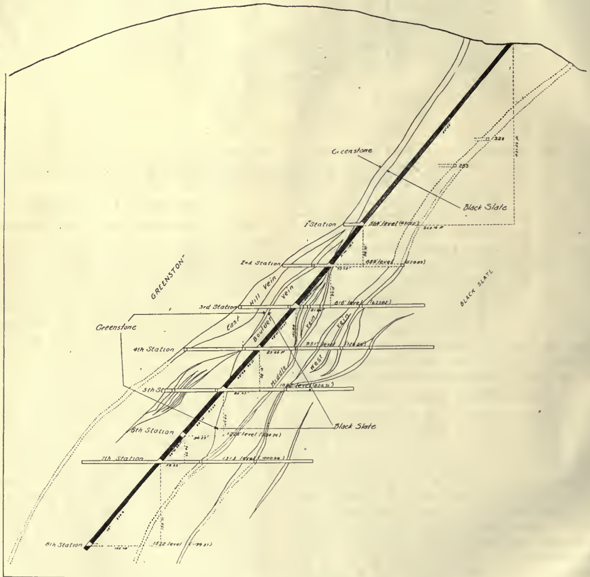
TYPICAL CROSS-SECTION, SHOWING BRANCHING OF THE LODGE.
